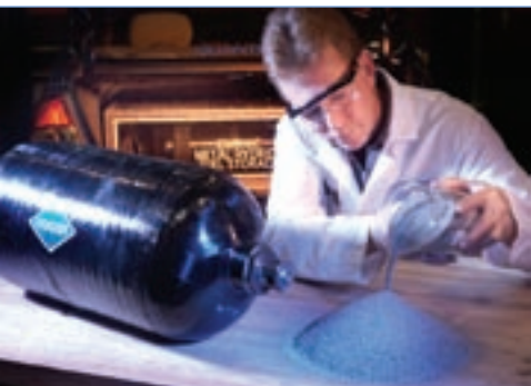
Solid Metal Hydride with Carbon Fiber Storage Vessel. Photo courtesy of ECD Ovonic
